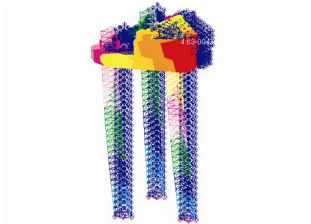
(a) Rolling vibration, f=0.104 Hz
