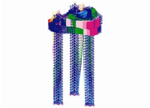
(c) Torsion vibration, f=0.115 Hz
