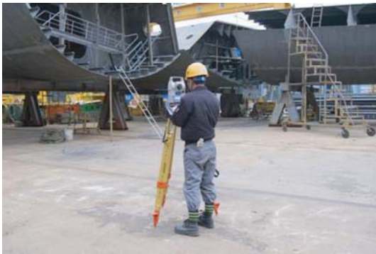
Fig.10 The measurement of ship block by the total station
