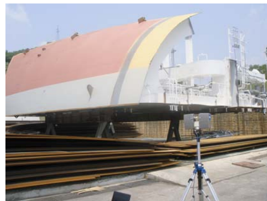
Fig.12 The measurement of ship block by the laser scanner
