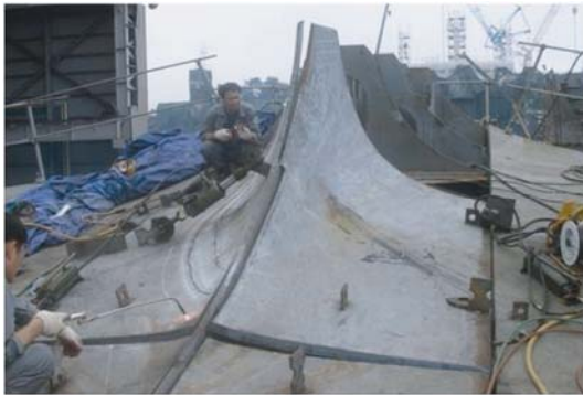
Fig.3 Line heating for modification of hull to close a gap between adjacent blocks
