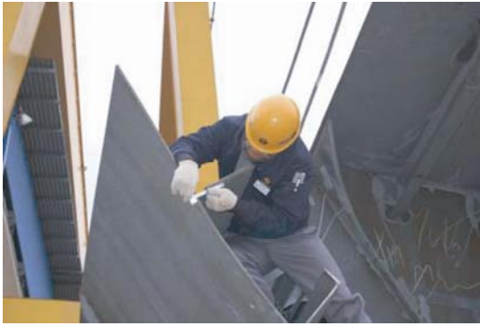
Fig.9 Put the sheet target for measurement by total station on the ship block
