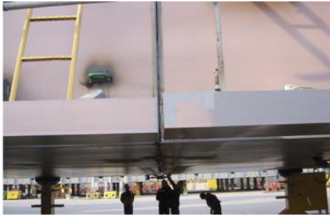
Fig.21 The blocks were erected at a time after simulation and cutting the blocks
