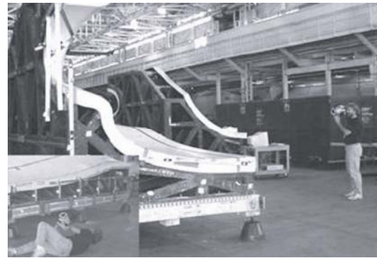
Fig.11 The measurement by photogrammetry system
