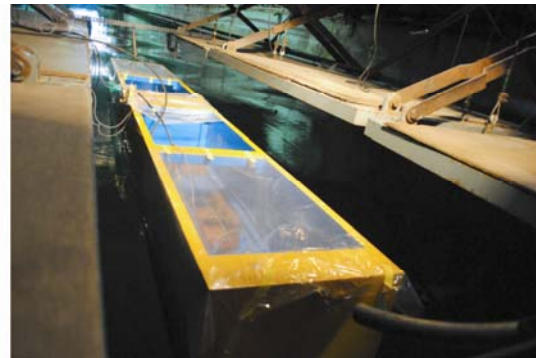
Fig.12 Scaled model hull in tank test
